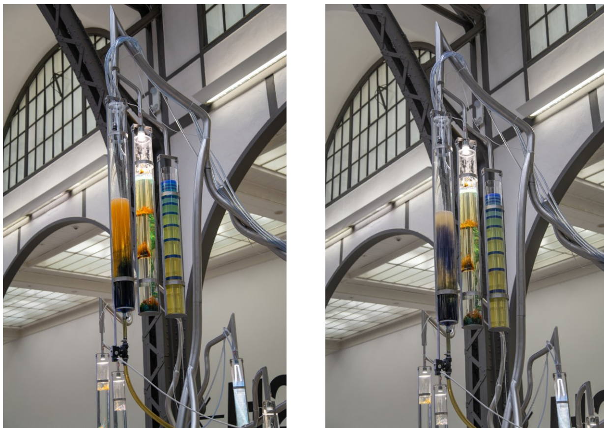
Figure 9. Live snapshots of the yellow-blue (left) and blue-colourless (right) transitions of the Briggs–Rauscher reaction.
