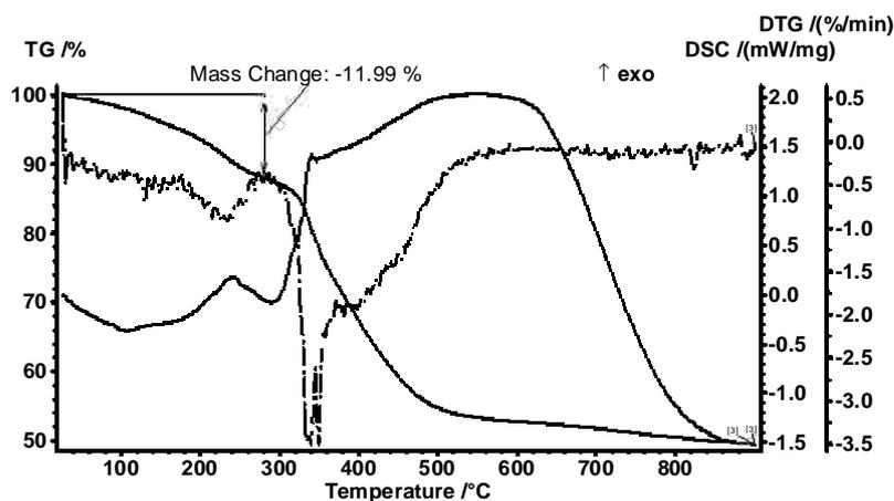
Figure II.15. TGA/DTG/DSC analysis of complex  $[\text{Cu}(\text{L}^1)_2(\text{H}_2\text{O})_2]$
