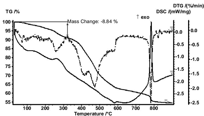
Figure II.16. TGA/DTG/DSC analysis of complex  $[\text{Co}(\text{L}^1)_2(\text{H}_2\text{O})_2]$
