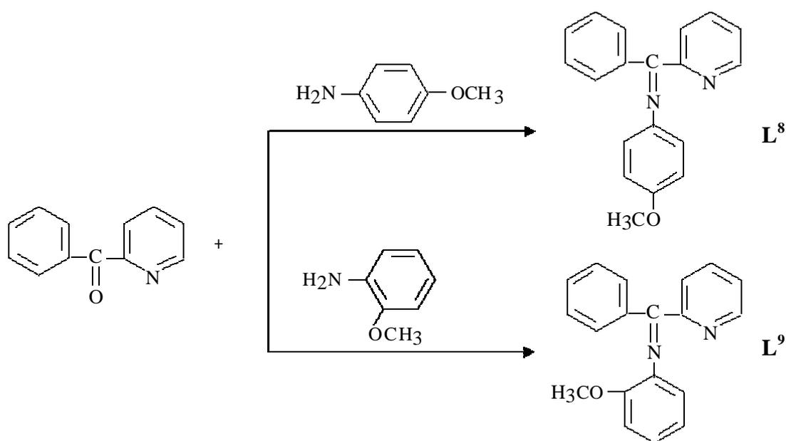
**Figure II.120.** Condensation reactions for the preparation of the Schiff-base  $L^8$  and  $L^9$
