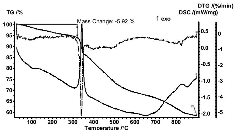
Figure II.18. TGA/DTG/DSC analysis of complex  $[Zn(L^1)_2]$
