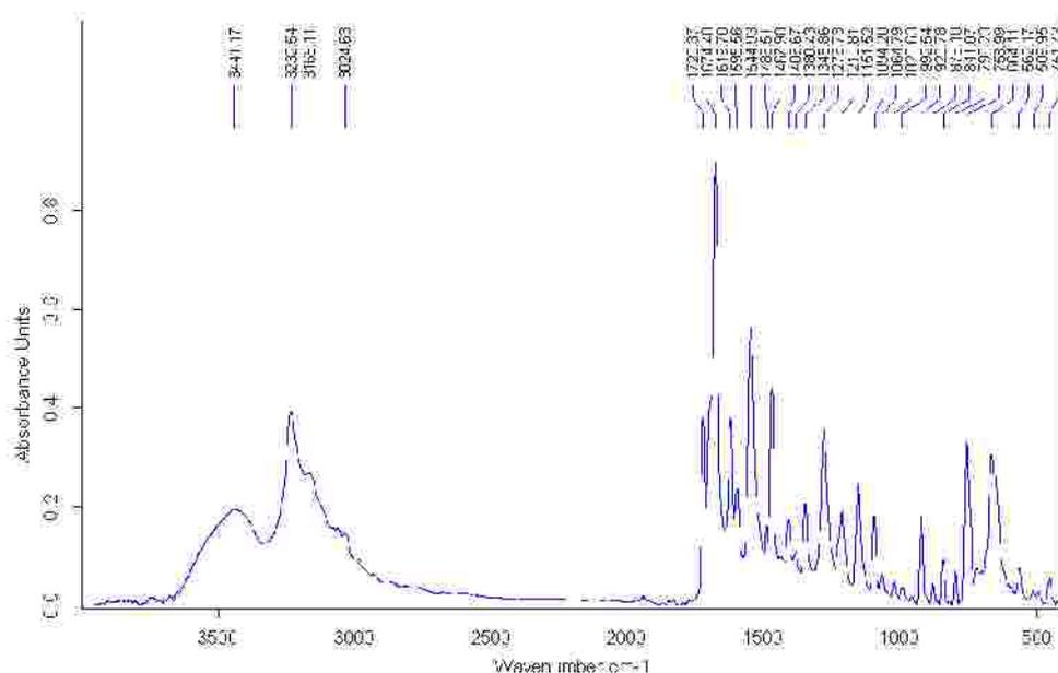
**Figure II.55.** IR spectrum of the Schiff base isonicotinoyl hidrazon-2 indolinone ( $L^4$ )
