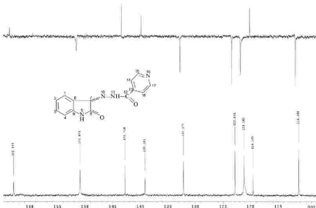
**Figure II.57.**  $^{13}\text{C}$ -NMR spectrum of ligand  $\text{L}^4$
