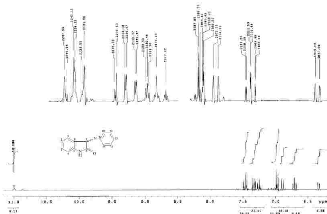
**Figure II.4.**  $^1\text{H-NMR}$  spectrum of ligand  $\text{L}^1$
