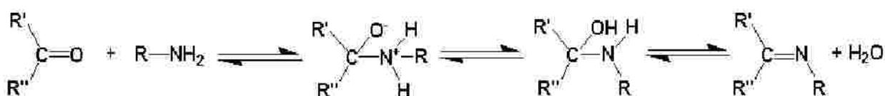
**Figure I.1.** Schematic representation of the general reaction for obtaining Schiff bases
