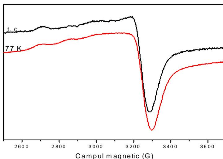
**Figure II.81.** EPR spectrum of complex  $[\text{Cu}(\text{L}^5)_2] \cdot \text{H}_2\text{O}$
