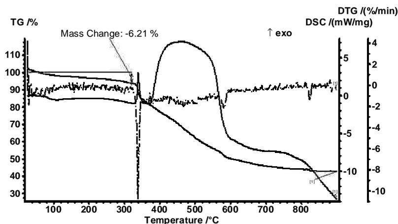
Figure II.19. TGA/DTG/DSC analysis of complex  $[Cd(L^1)_2]$
