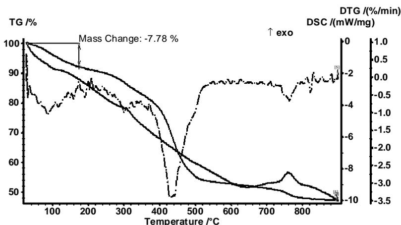
Figure II.17. TGA/DTG/DSC analysis of complex  $[\text{Ni}(\text{L}^1)_2(\text{H}_2\text{O})_2]$
