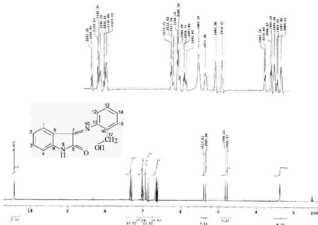
**Figure II.72.**  $^1\text{H-NMR}$  spectrum of ligand  $\text{L}^5$
