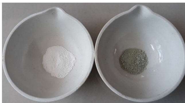
Figure 18. ZrO 2 -SO 4 (left) and Cr/ZrO 2 -SO 4 (right) catalyst. Reprinted with permission from Dr. Hauli, Ref. [71].
