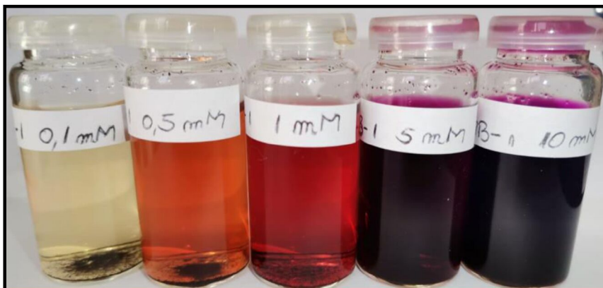
KMnO 4 solutions after 24h of contact with MB-1
